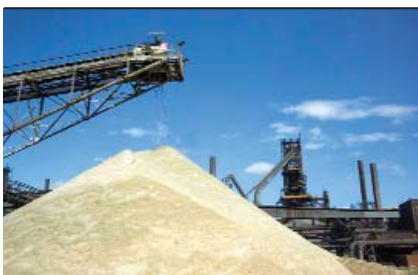
Left: Our granulated blast furnace slag is used as a valuable secondary material in the cement industry.
