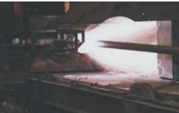
Aluminium spraying on automatic equipment.
