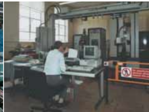
Automatic tensile testing of Tube Feedstock.
