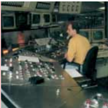
Control cabin of electric welded stretch reduction mill.
