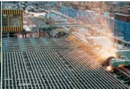
Hot Finished Tube on cooling beds.
