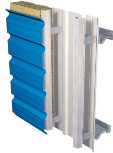
Horizontal wall (HW) systems include Tata Steel's vertically laid liner on standard horizontal secondary cladding rails. With an Instaloc® HW spacer system which spans easily between the support points to carry a range of standard horizontally laid external trapezoidal, plank and sinusoidal profiles. These options can be expanded upon using our additional range of special profiles, providing a unique look for any project.
