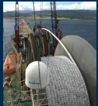
CSO Apache vessel begins spooling of pipe ready for pipelay
