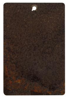
Mild steel corrosion coupon underneath PV panels showing heavy red rust and flaking.
