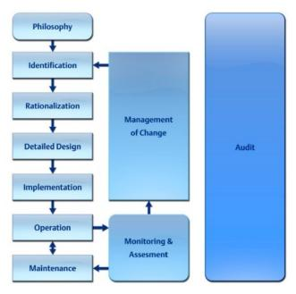
The alarm philosophy constitutes the first step in the "Alarm Management Lifecycle" process. It is important to determine first what an alarm is.
