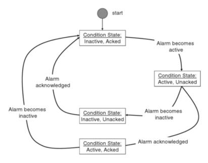
By using buttons on the HMI screen or alarm list, alarms can be acknowledged (acked). Often there is a separate button to turn off the sound after a new alarm has occurred. The acknowledge button has the same function. Per alarm class (§1.4) can be set if an alarm must be reset manually or if this is done automatically. For alarms with class PRO the operator shall always acknowledge manually (see §1.2 point 1).
