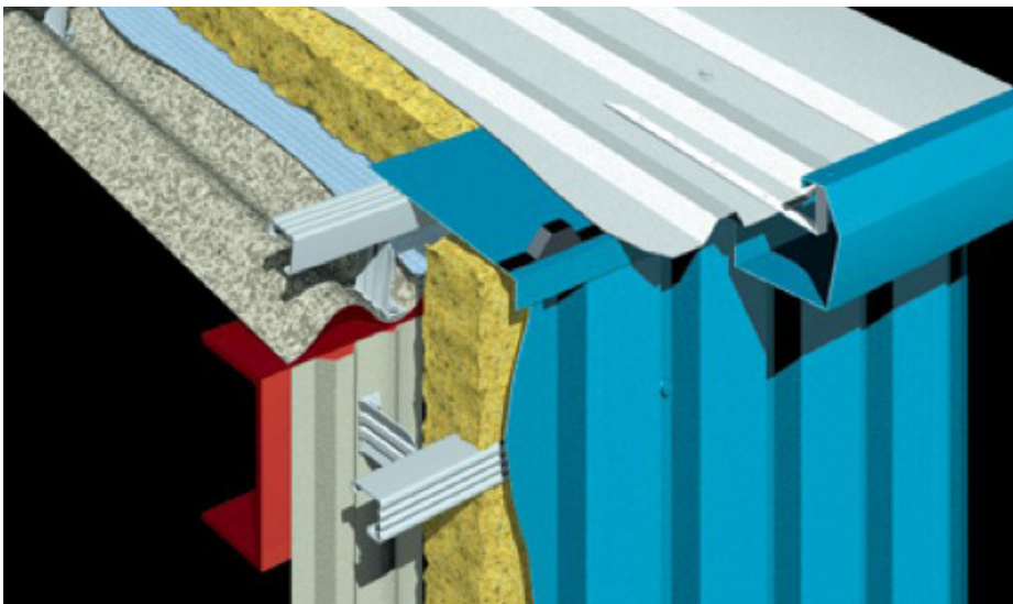
Figure 8. Through fix pre-finished steel profile insulated over cladding system
