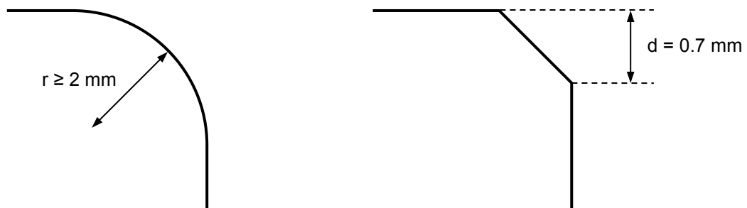
Figure 1: Minimum size for rounding or bevelling corners and edges in accordance with ISO 8501-3 §2.2 and ISO 12944-3.
