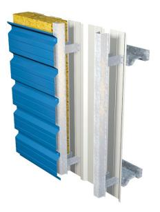
Horizontal wall (HW) systems include Tata Steel's vertically laid liner on standard horizontal secondary cladding rails. With a spacer system which spans easily between the support points to carry a range of standard horizontally laid external trapezoidal, plank and sinusoidal profiles. These options can be expanded upon using our additional range of special profiles, providing a unique look for any project.
