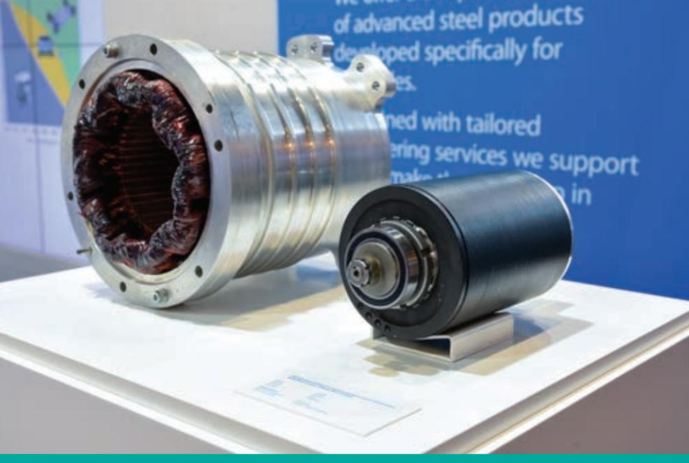
Motors with high power and torque densities achieved at high speeds are tough on materials, so they need steels that combine good magnetic properties with resistance to stress (Courtesy of Tata Steel Europe)
