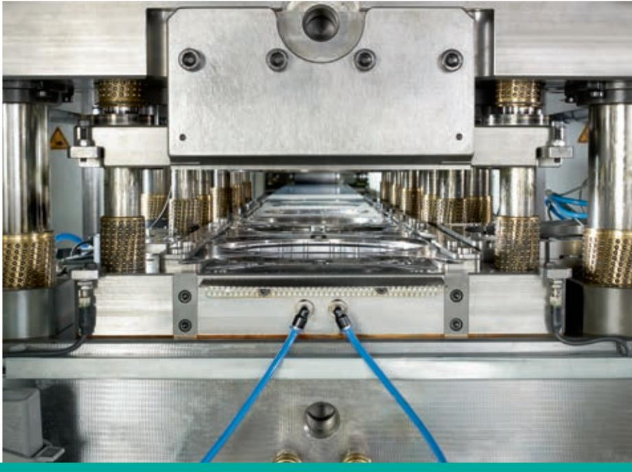
A production station for a cold-stamping process for lamination stacks, which combines prime electrical steel with a full-face bonding process (Courtesy of Voestalpine Automotive Components Nagold)
