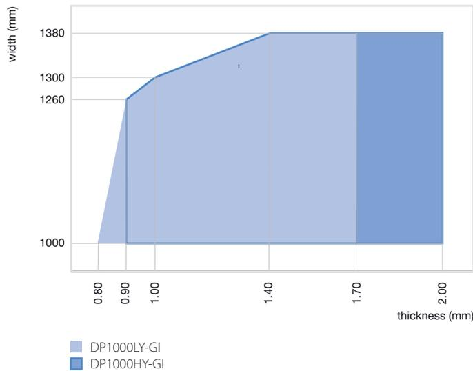
Mechanical and dimensional properties are according to VDA 239-100 requirements. Please contact us for other dimensions.
