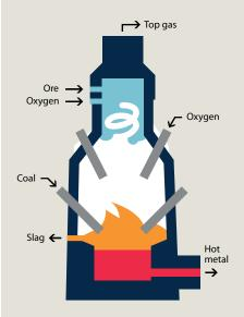
HIsarna consists of a reactor which maintains a temperature above the melting point of iron throughout, so that the injected iron ore immediately melts and is converted into liquid hot metal. The very high temperature of the process gases in the melting vessel is further increased in the cyclone at the top of the reactor by the addition of pure oxygen, which reacts with the carbon monoxide present.
