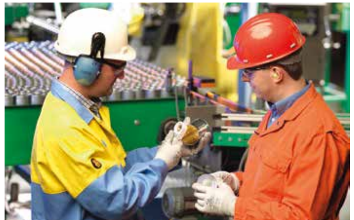
The D&I canmaking line at Tata Steel's R&D facility is run at commercial speeds. In co-operation with customers, it offers the opportunity for development of the canmaking process for 2-piece D&I food cans using Protact laminated steel.
