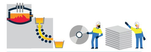
Through EAF steel production, new steel can be made with scrap steel. This significantly reduces energy use and the reliance on raw materials. Each item of recycled steel saves one and half times its weight in CO<sub>2</sub>.
