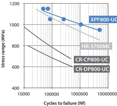
Figure 3: S-N fatigue curves (R = -1) of XPF800-UC in comparison with hot-rolled S700MC
