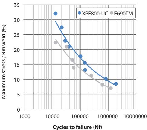
Figure 4: S-N weld fatigue curves (R = 0.1) with lap shear loading configuration based on GMAW arc welding of XPF800-UC compared with E690TM. Plotted vertically is the maximum stress divided by the tensile strength (3xHV) of the weld. Filler wire used: ER120S for XPF800-UC and E690TM
