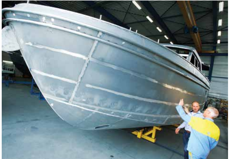
The hulls of Linssen's motor yachts are particularly smooth thanks to Tata Steel's S235.
