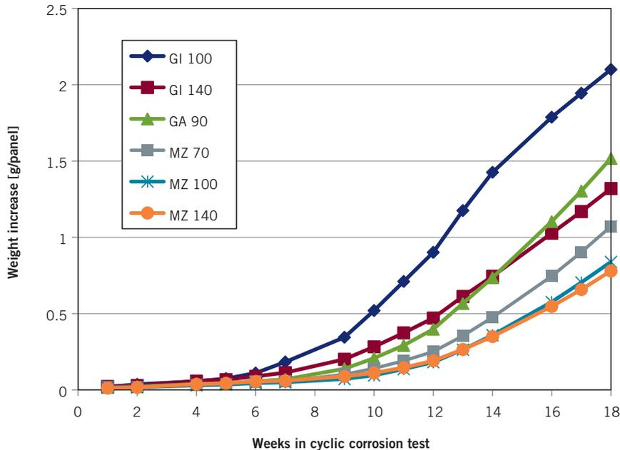
5 Weight gain of panel by red rust during glass flange test (Volvo design)
