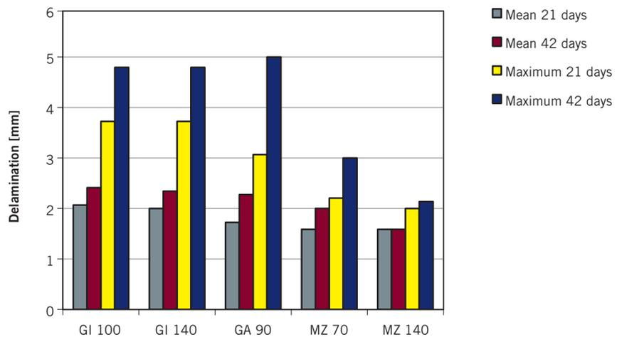
③ Scribe delamination in ECC1 cyclic corrosion test with average and maximum values after 21 and 42 day cycles
