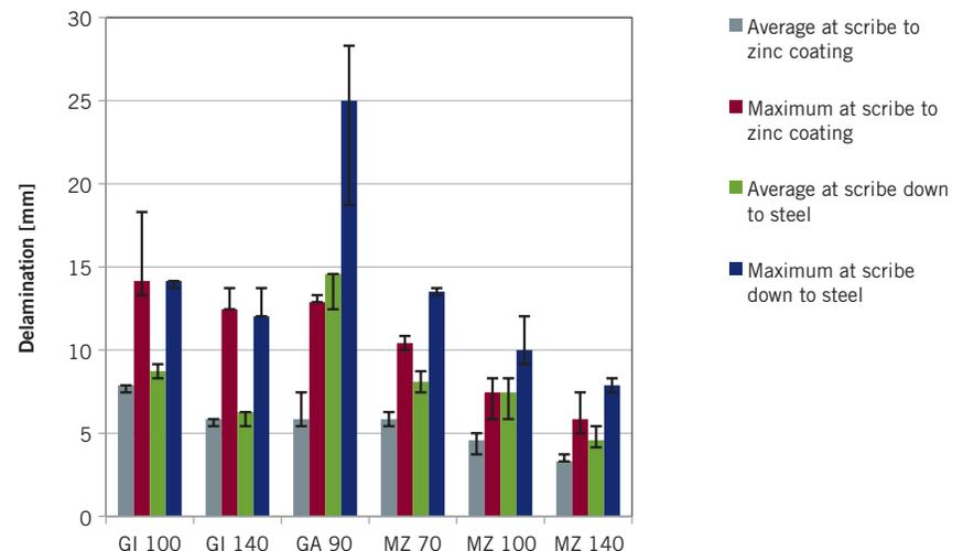
④ Average and maximum scribe delamination values after 20 weeks, with scratches down to the zinc coating and scratches down to the steel substrate
