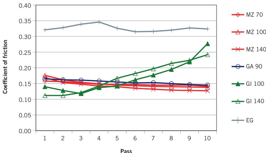
2 Linear Friction Test results show the development of friction and material damage due to the adhesion of zinc on the tools
