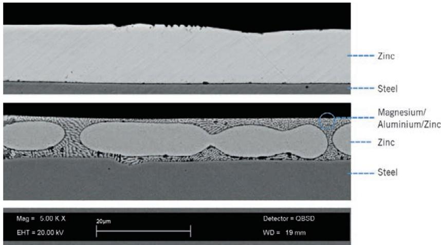
1 Cross-section of microstructures: pure zinc coating (above), MagiZinc coating (below)
