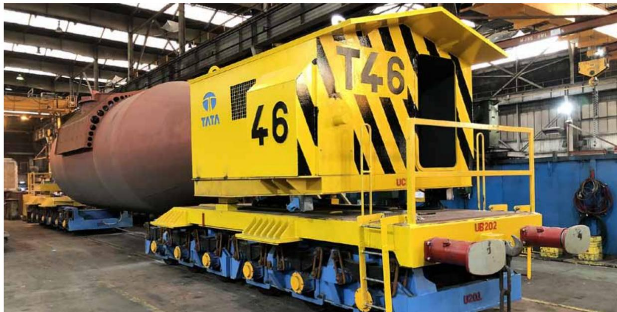
Torpedo 46 transports liquid iron between the blast furnaces and BOS Plant
