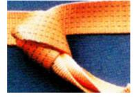
Never use with knots. Knots can reduce the capacity by a half.
