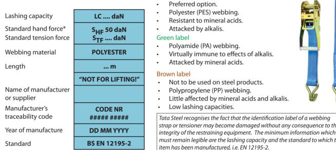
\* An applied force of 50kg (daN) to the handle, will typically result in 350kg (daN) of tension in the lashing.
