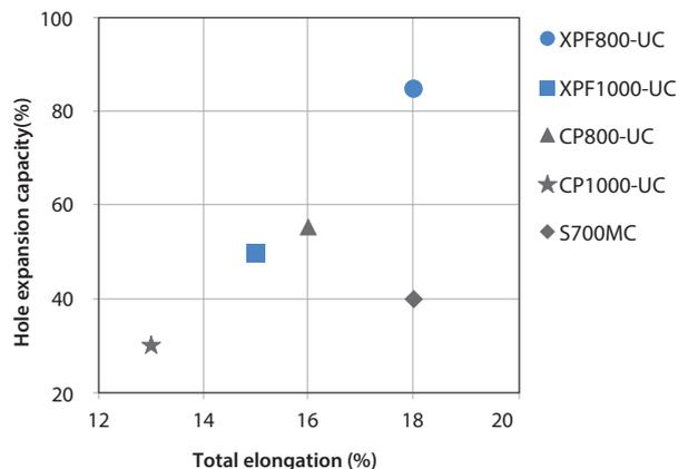
Figure 2B: HEC versus total elongation for XPF800-UC from laboratory trials
