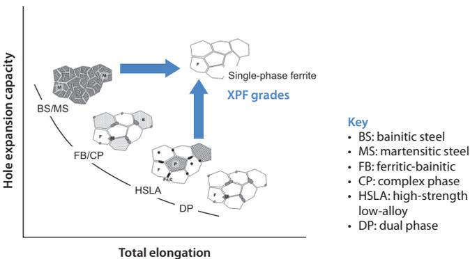
Figure 1: A key measure of the formability of steel is hole expansion capacity (HEC) – how far the material around a stamped hole will stretch before fracturing. XPF combines the hole expansion performance associated with bainitic and martensitic grades, with the elongation characteristics of dual phase (DP) and high-strength low-alloy (HSLA) steels
