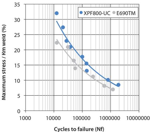
Figure 4: S-N weld fatigue curves (R = 0.1) with lap shear loading configuration based on GMAW arc welding of XPF800-UC compared with E690TM. Plotted vertically is the maximum stress divided by the tensile strength (3xHV) of the weld. Filler wire used: ER120S for XPF800-UC and E690TM
