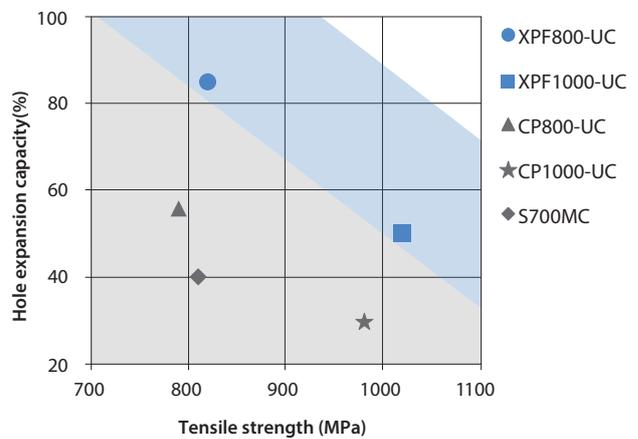
Figure 2A: HEC versus tensile strength for XPF800-UC from laboratory trials
