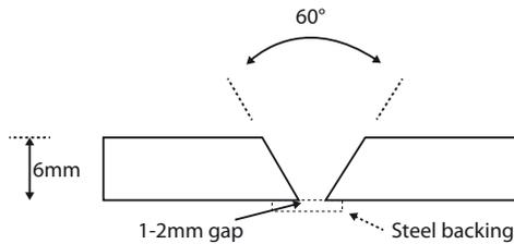
R&D weld test setup: Nil pre-heat, max interpass temperature 68°F. Union X96 wire (1.0mm), M21 gas 80/20
