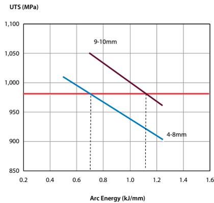
Plot of UTS vs arc energy resulting in recommended heat input
