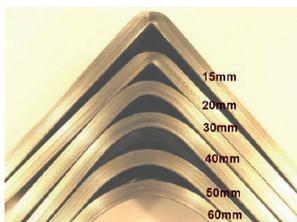
Bend samples for 6mm gauge resulting in guaranteed minimum inner bend radius
